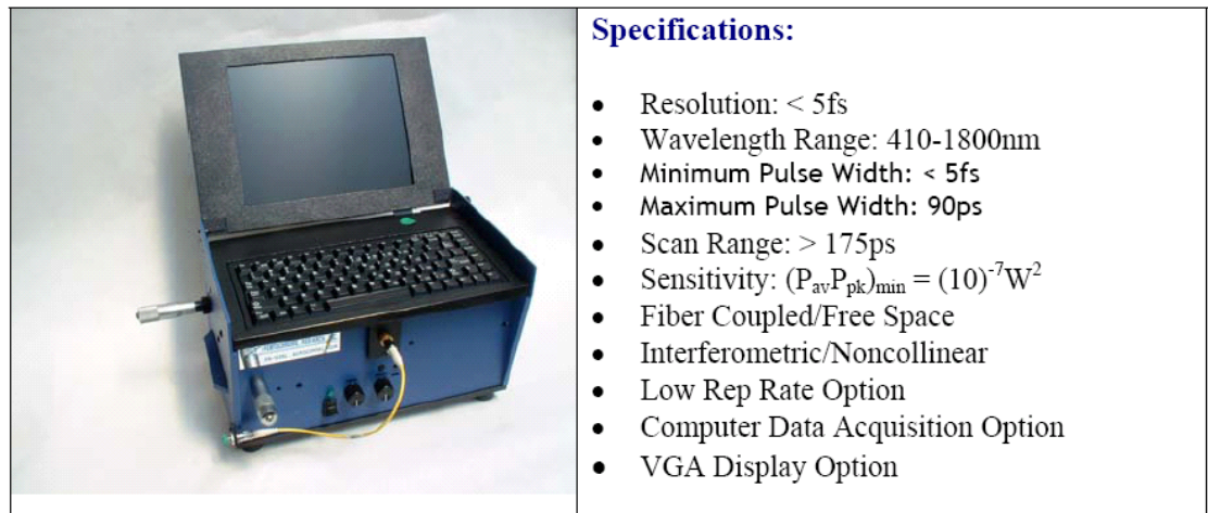
Figure A-2 specifications of the model FR-103XL rapid scanning autocorrelator
